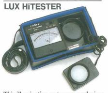
This illumination meter uses a selenium photocell in the receptor, matched to a high-sensitivity meter. The highperformance internally magnetized taut band meter is designed for on-side environmental measurements, backed up with visual sensitivity and angle compensation. Ideal for illumination measurement in offices, factories and hospitals.
