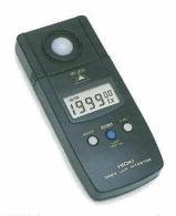
The 3423 is an easy-to-operate handheld unit that can measure a broad range of luminosities, from the low light provided by induction lighting up to a maximum intensity of 199,900 lx.
